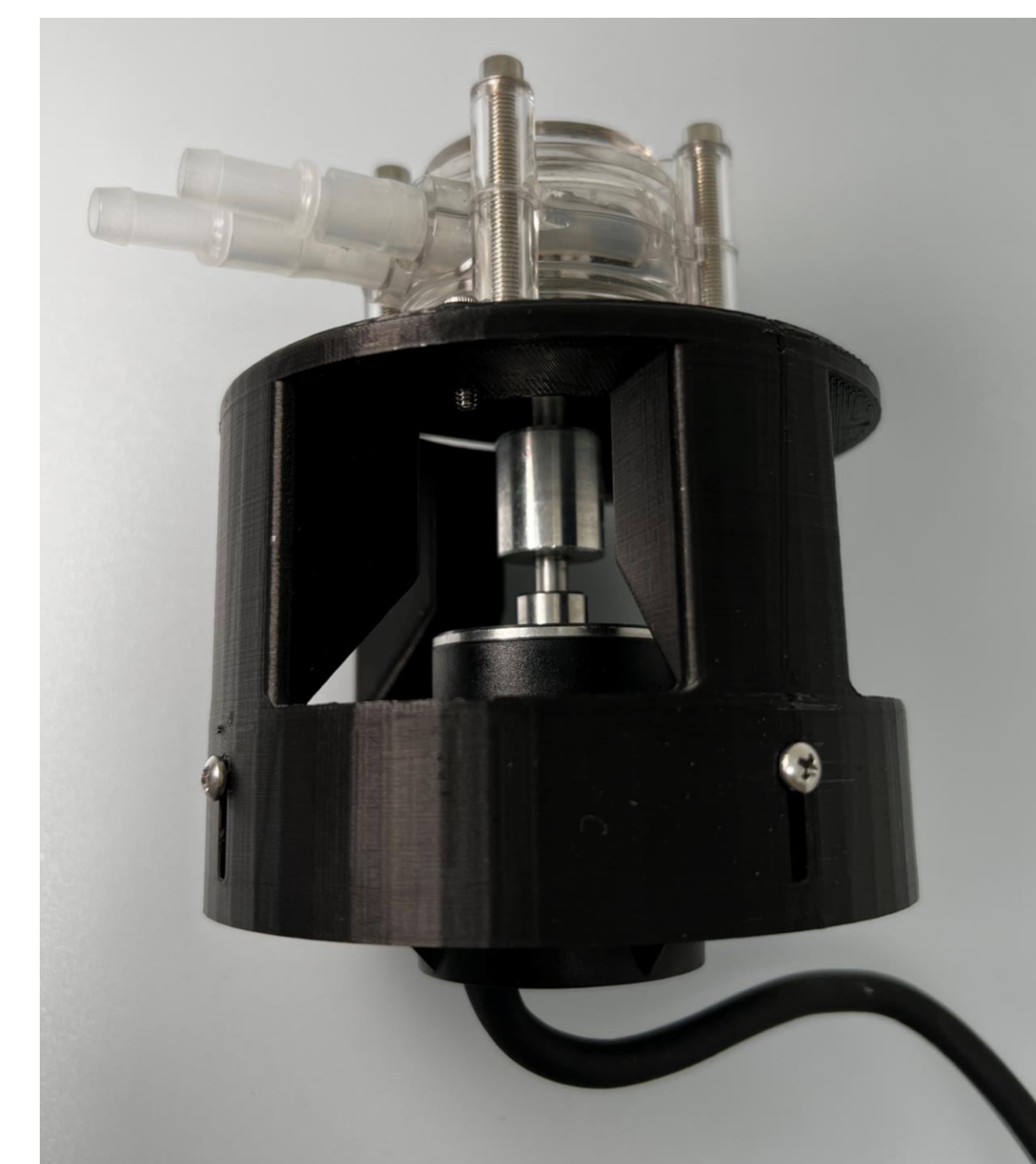
Close up of peristaltic pump connected to submersible motor
