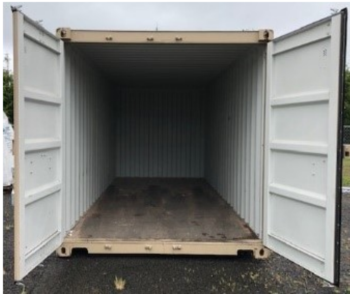
Figure 10: Shipping Container with Wood Floor
